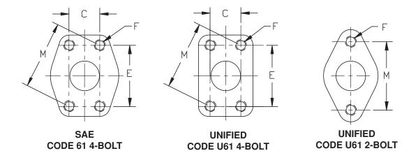
Unified Code U61 2-bolt flange ports may be nested together even more closely than their 4-bolt U61 counterparts. When the U61 2-bolt ports are utilized with **Adaconn®** Unified Code U61 one-piece, two-bolt flange adapters, they may be qualified at working pressures similar to the maximum working pressures of comparably sized SAE Code 61 split flange applications. This gives the designer a means to minimize the size and weight of hydraulic components.
