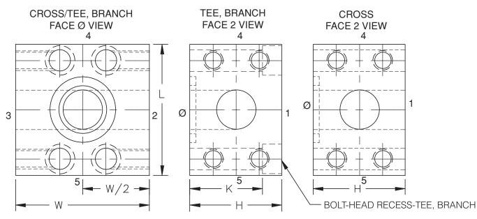
DESIGN A = AS SHOWN on drawings above and the title block schematics below. DESIGN B = Eliminates seal groove and O-Rring from Face- $\emptyset$ .
